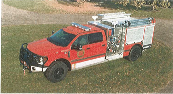
Example of NFPA 1901 minimally compliant fire engine to meet minimum ISO fire apparatus requirement
